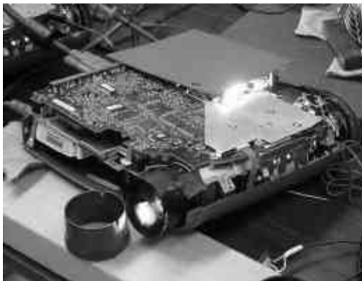
Modified single chip DLP projector
