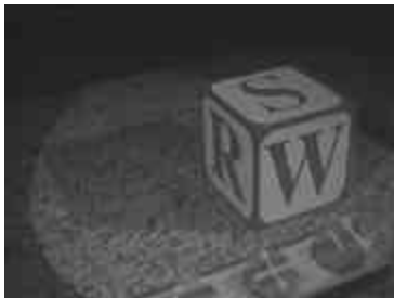
Image seen by a head tracked user standing to the left of a cube located on the surface of the bench display.
