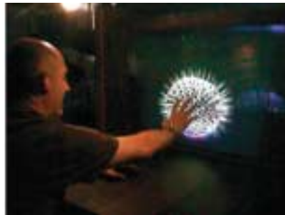
(a) (b) (c) 3 Creating a virtual workspace: (a) a holographic diffuser allows simultaneous viewing of projected and real images; (b) shared virtual workspace projected between collaborating users; and (c) four-person configuration.
